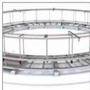
Frames guide and protect the chains. The bottom plate is designed to avoid accumulation of coal or other dirt.
